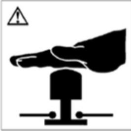
When the forklift is in a variety of emergency situations, the emergency stop button should be pressed immediately.
